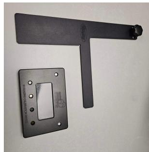
Calibration device and plate holder. Used to center device and well plates, Plate holder connects on the pins to the left
