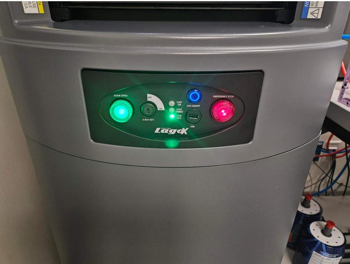
On the LagoX, the green button on the left will raise the door. In the center is the X-ray indicator lights. The red button on the right is the emergency stop button.
