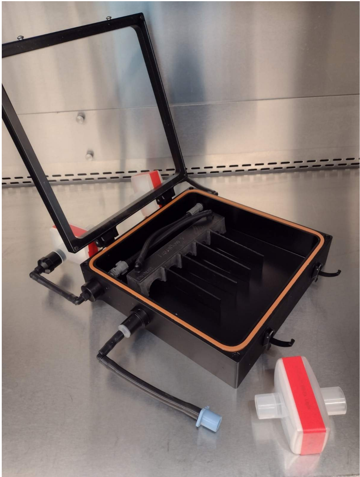
BSL-2 IVIS imaging box open inside a biosafety cabinet
